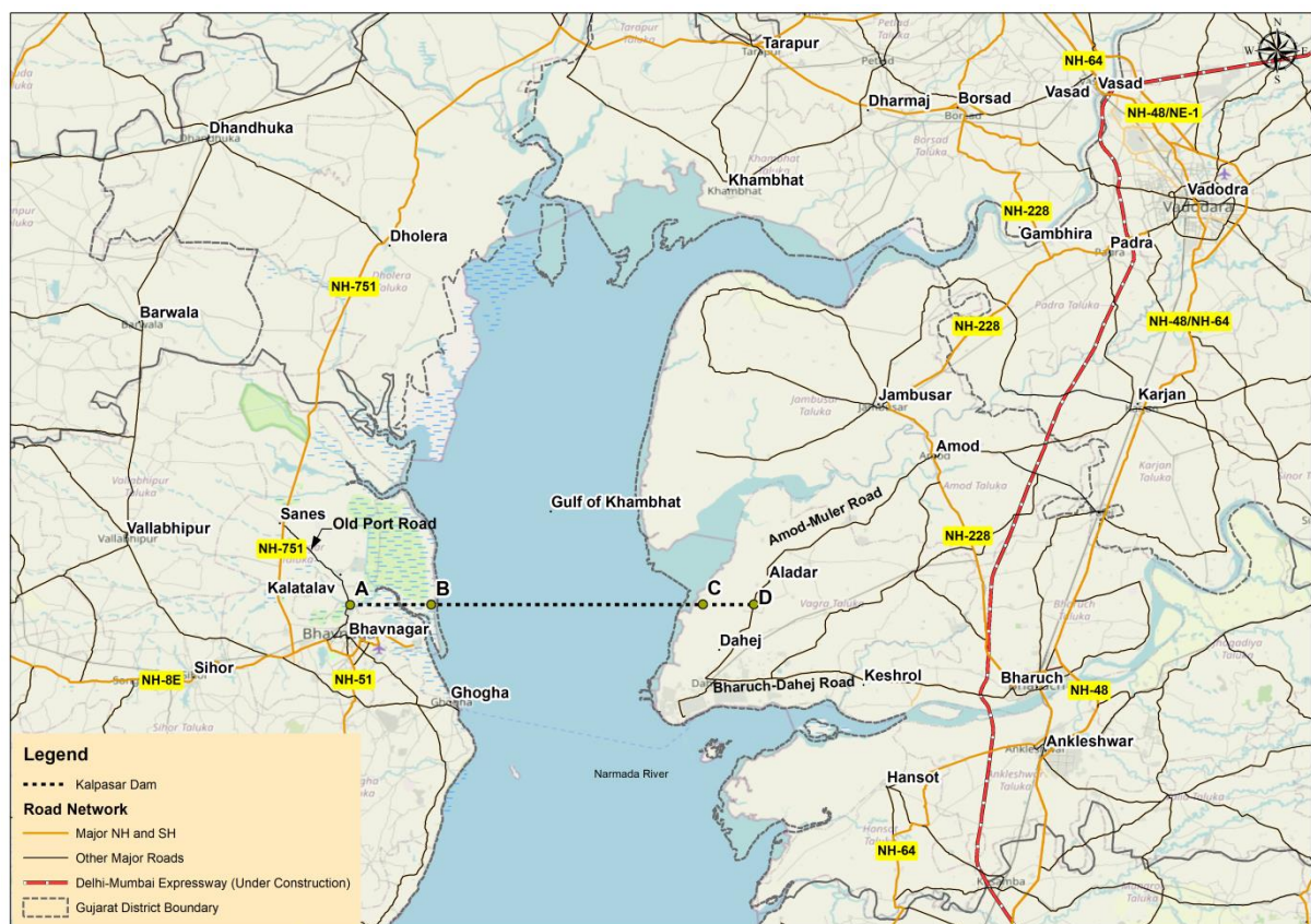
Figure 2.66: Alignment of Kalpasar dyke and access roads
